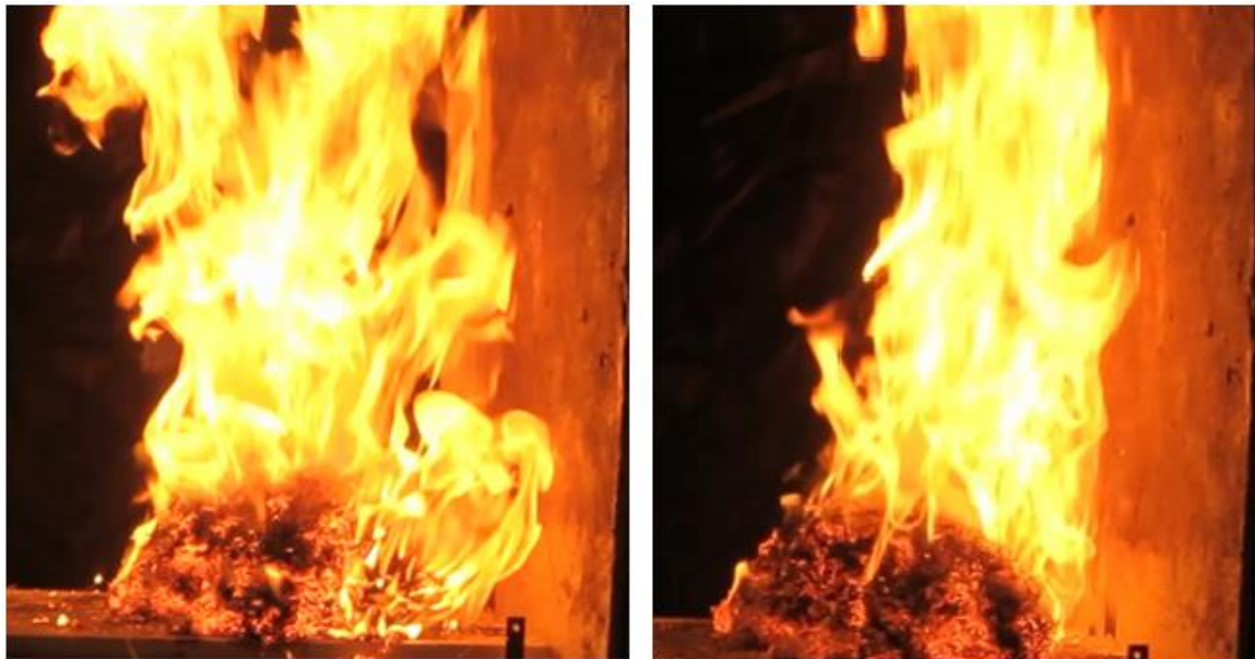
Figure 2.15 Burn #3 and #4 with Figure 2.12 configuration exhibiting flame tilting at a critical distance (left) and fire touching wall towards the end of burn(right).
