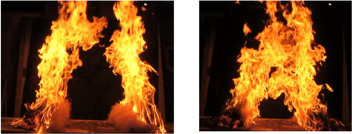
Figure 2.16 Burn #5 with Figure 2.13 configuration exhibiting flames seeing each other at a critical distance (left) and merging, creating junction zone (right).
