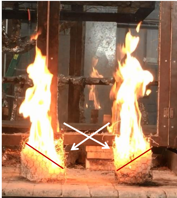
Figure 2.5 Burn #6. Sloped burnt fuel is noticeable. White arrows mark the radiant preheating of the fuel
