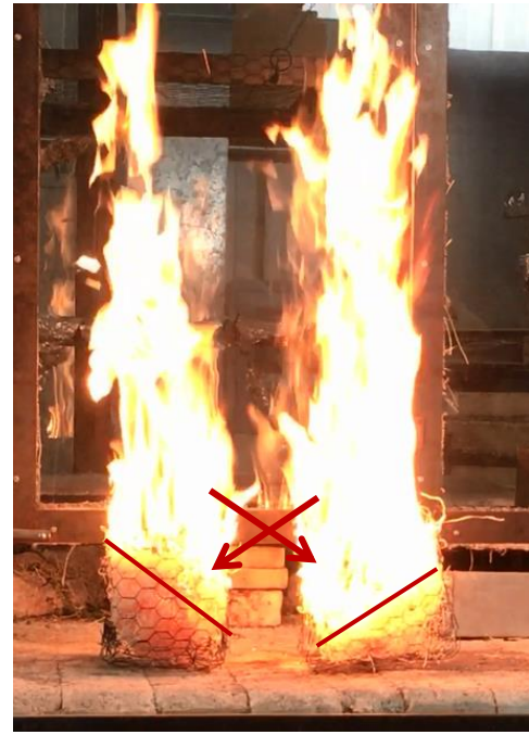
Figure 2.6 Burn #7. Sloped burnt fuel is noticeable. Red arrows mark the radiant preheating of the fuel
